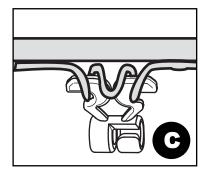
Twist "body" of clip slightly again to spread "arms" of clip. Clip "arms" must be flat and touching edge to edge as shown, not overlapping.
